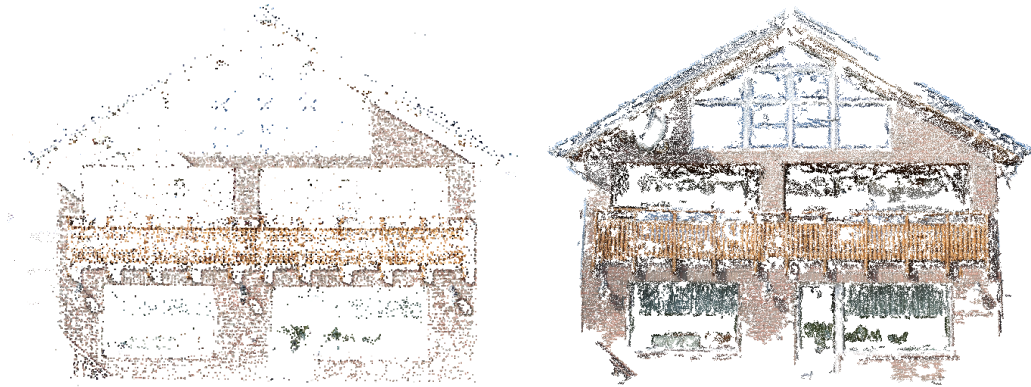
Figure 2.7: Comparison of a sparse reconstruction point cloud (left) and a dense reconstruction (right) of a building front. The example has been created using the Bundler SfM software [Snavely 2006] and PMVS2 [Furukawa 2010b] from a dataset of 29 images.
