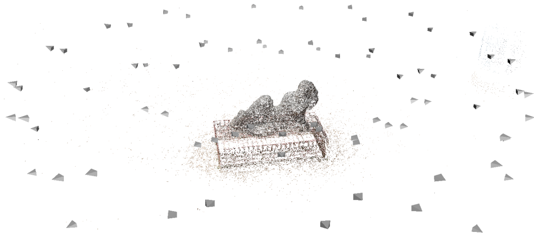
Figure 6.1: Visualisation of the sparse reconstruction of the “Der Hass” dataset by [Fuhrmann 2014]. It shows the sparse point cloud as well as estimated camera positions, which can be selected for display separately.
