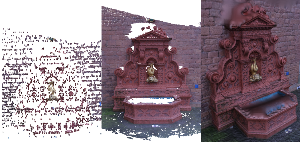
Figure 6.2: From left to right: Sparse point cloud, dense point cloud, surface reconstruction of the “fountain-P11” dataset by [Strecha 2008].
